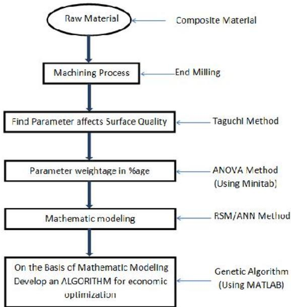
Above optimization algorithm of modeling and determination of optimal or near-optimal cutting process parameter conditions, may be give interesting result in end milling machining process development of composite material cutting operation.
